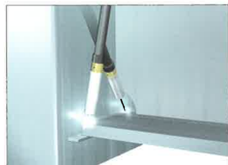
▲ for Fillet welding in a tight space
